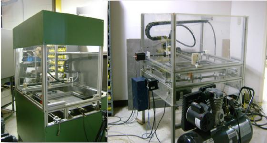
Fig. 1. Two views of the XY plasma cutting machine
