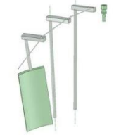
VIGV Lever arms actuation arrangement
