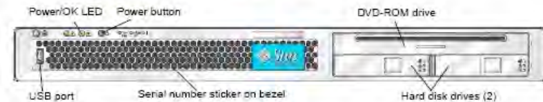
FIGURE 1-1 Sun Fire X4100/X4100 M2 Server Front Panel
