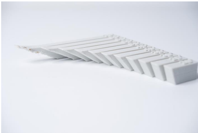
Figure 6 Overhang example ( https://www.3dhubs.com/knowledge-base )
