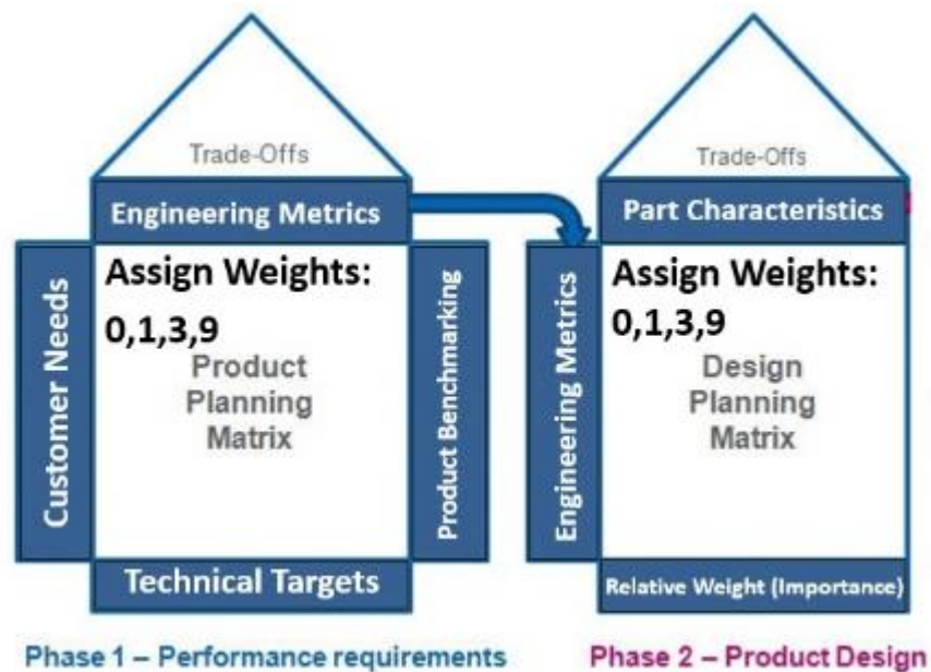
Figure 5 – Example of a QFD Phase I & II diagram in abstract form. This is shown to simplify the intricate spreadsheet that is used for QFD analysis.
